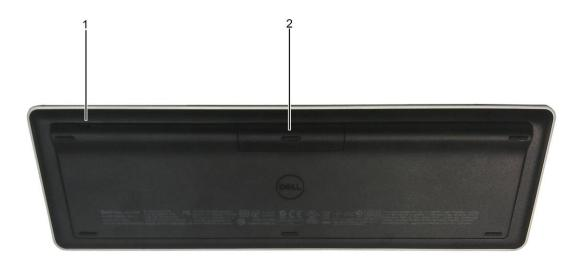
1. Power switch 2. Battery compartment
